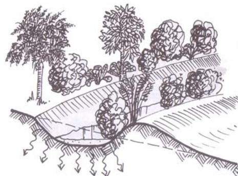
Figure 4. A swale where water is retained and used efficiently by the crop. Andrew Jeeves, 1988.
